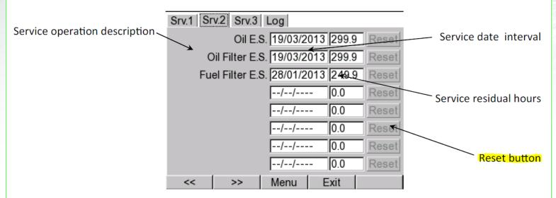
After the service operation has been performed the number of hours counter and date interval must be reset to original value by pressing the corresponding Reset button. The Service or Factory login allows to activate Reset buttons. The unit also records each reset operation with date time in a special log file.
