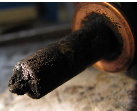
Figure 3, Injector with carbon deposits from unburned fuel
