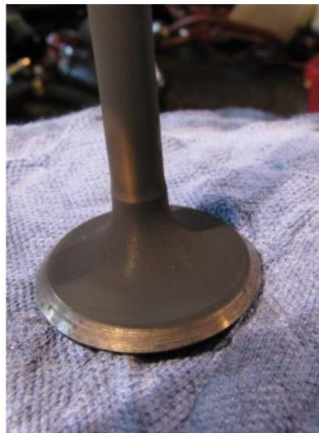
Engine tested with load (exhaust valve)
